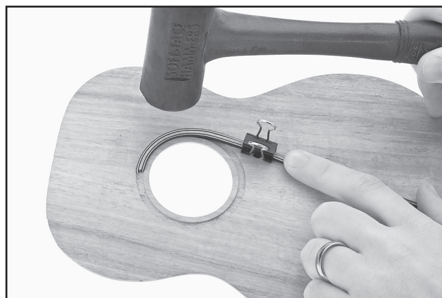
Figure 8. Installing the purfling.
